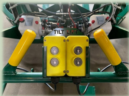
Controls to lift & tilt without removing hands from steering handle
